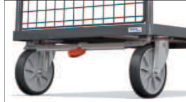
TOTALSTOP - the fetra central brake system With only one foot the rotation of wheels and the swivelling movement of both swivel castors can be securely locked. The brake pedal is always visible to the operator. Standard with TOTALSTOP.
